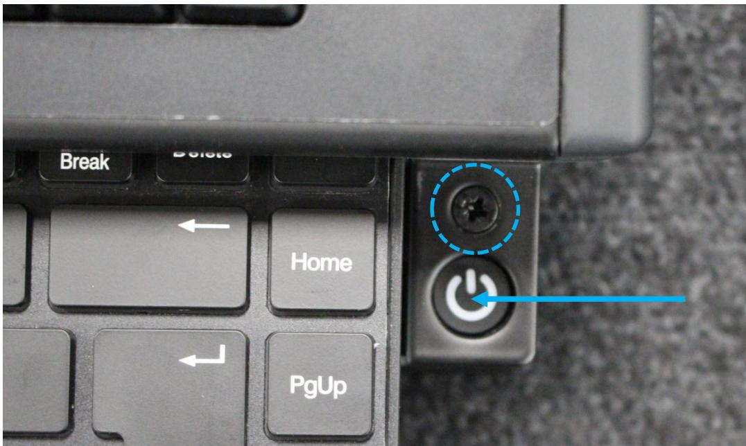
c. Fix the Program Panel with M4 black screws under the left hand side trim
