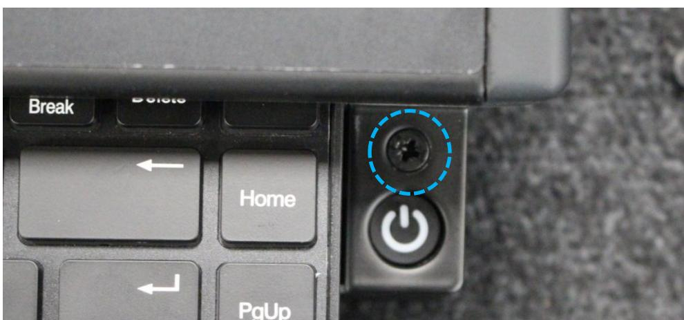
c. Keep the keyboard drawer opened then secure the Program Panel on the Panel stay
