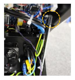
c. Disconnect and discard the 2x 3way mascon connectors orange/black loom.
