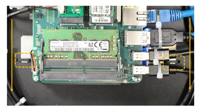
Fix the PC frame with retained 2x M3 nuts and M3 washers
