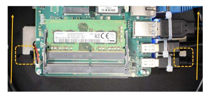
Remove the PC frame from the 2x studs then move it about 20mm to the right for getting access to USB port on motherboard.
