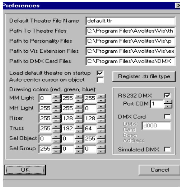
This dialogue allows selection of paths to theatre files, personality files, personality extension files, and DMX reader card firmware files. These should be changed with caution. If set incorrectly, the Visualiser will not be able to locate these files, and will not function correctly.
