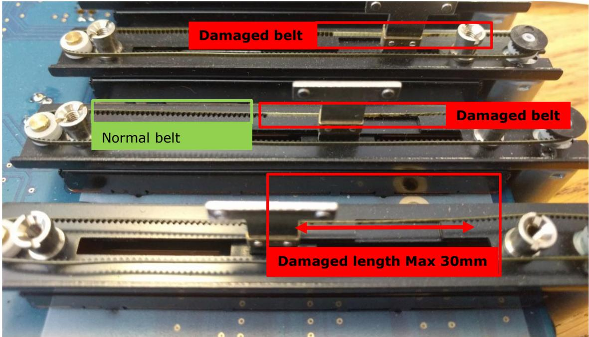
Check that the belt wear is not too long, the maximum damaged belt length is 30mm
