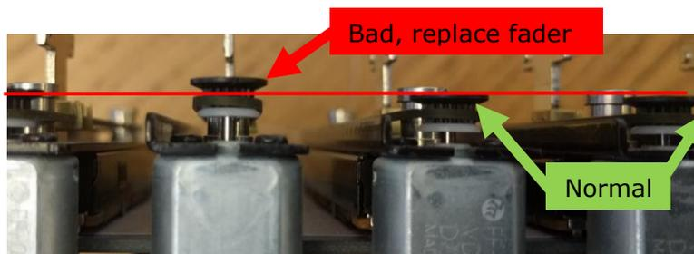
4. Replace the fader if the pulley has moved up
