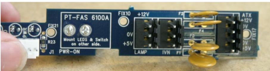
Remove and discard the F3 fuse, and open the hole near the "INV" connector.
