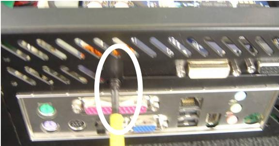
4. Slide the Interface to the left and fold it away to get access to the dongle.
