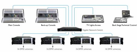
Networking of the outputs using the TNP increases system capabilities to up to 64 DMX universes, catering for even the largest world class spectaculars. All of this can used in conjunction with Titan Remote!
