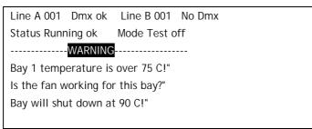
Ensure that all fan vents are clear and that sufficient air flow is available to naturally cool the module.
