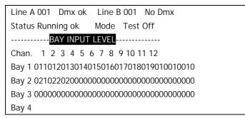
The screen shot above shows a 48 way frame with three 12 channel dimmer modules fitted.
