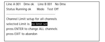
Use the UP and DOWN buttons to select the desired limit, then press Enter.
