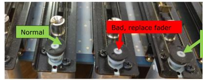
Normal, shaft 0.5mm Below pulley
