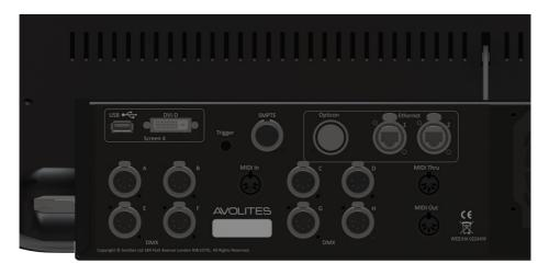
All the connections required for the console are found on the back panel.
