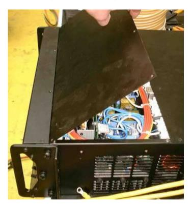
Check that both strips have "stuck" to the cover before finally fixing the cover to the dimmer.
