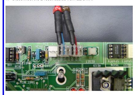
2. Solder the 2 off 3 way MAS-CON headers (supplied) 'back to back' so that they provide a path to link the 2 connectors removed in step 1.
