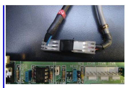
5. Cable-tie the assembly to the loom.
