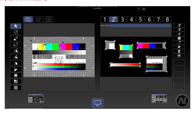
The screen fixture provides an underlying toolset to allow you to create regions, specifying an area on the output to draw to, and what part of the texture to extract from. Where the main unit of control here will be pixels. If a region has inequality between the sizes of the source and destination, then Ai will perform bi-linear interpolation for the scaling. Scaling linearly in both the width and height.
