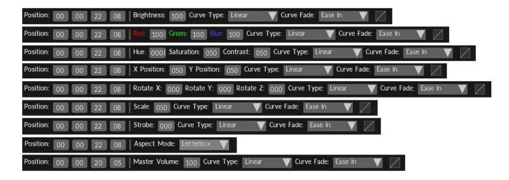
Above we can see which parameters are available for each video attribute type when selecting the relevant keyframe on the timeline. Starting at the top and working down we have Brightness, RGB, HSC, Position, Rotation, Scale, Strobe, Aspect Mode and Master Volume. Each marker type has it's own unique set of parameters, however all of them start with the time in H:M:S:F. at which the keyframe occurs and all of them end with easing curve options.
