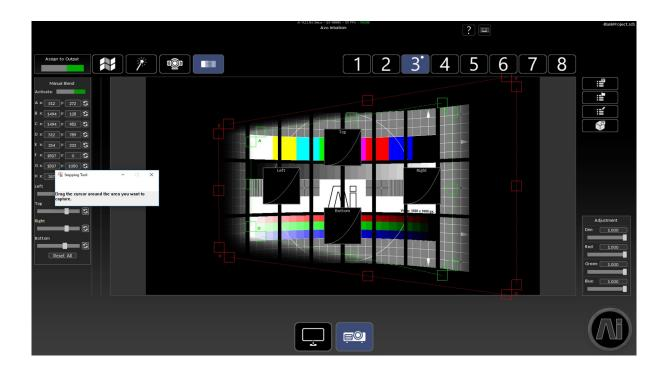
In previous versions of Ai, softedge blending was accessed via the Projector Output Page. Version 11 introduces a separate page for controlling blending which can be accessed from the new icon at the top of the Projector Output Page alongside the icons for Autoblend and Automap.
