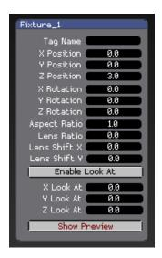
The projector fixture should be used when you intend to do video mapping or vertex editing using a 3D model. It works in conjunction with the Screen Fixture models, by capturing their geometry and then applying adjustments on those based on it's positioning in the Virtual Scene.
