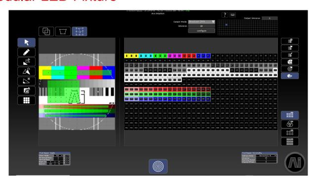
The modular LED fixture takes a similar approach to the Screen fixture for mapping information to an output using regions. However instead of a source and destination, there is only a source to be drawn. Where the destination is defined using a channel grid for the ArtNet data. You can define the current universe that the region is on, with the starting channel. Depending on the definition of the region the output page will calculate the pixel information to be sent over DMX.
