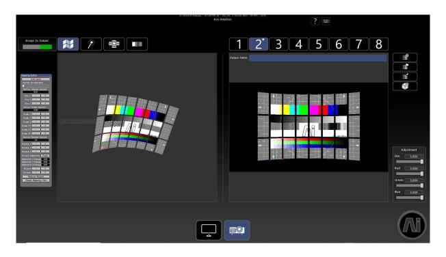
The projector fixture operates differently to the other two fixtures, where there is no region data used for the mapping. However it still follows the source and destination principles. Instead of using regions, it will use the 3D geometry data of the models loaded onto the various screen fixtures that it can see. You will then see a preview of the output, which is a snapshot of what the projector can see from the virtual scene.
