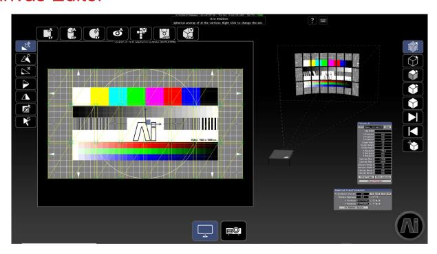
When making use of a 3D model for a screen, there are two important parts to the process – the 3D geometry of the model itself and also how your image is applied to this geometry, also known as the UV Map. UV mapping is a term used to describe the process of placing your screen shape within a defined texture area and generating coordinates for it based on this information. The U and V are used to mean horizontal and vertical as X and Y are already used for referring to position.
