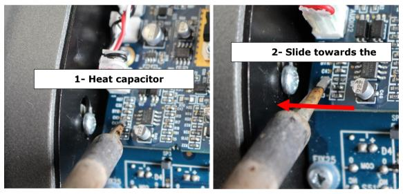
Make sure that the capacitor is removed from the board,
