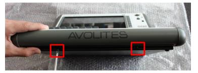
Open up the front panel and secure using the stand (right hand side), the stand engaged in to the side of the front panel.
