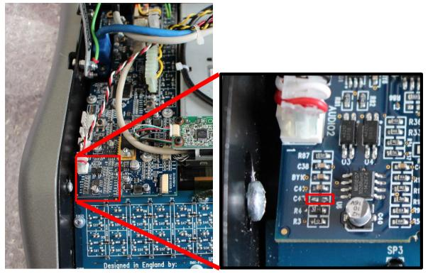
Using a soldering iron remove this capacitor,
