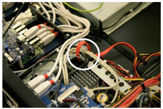
Disconnect the power and SATA cables from the rear of the optical drive. Remove the SATA cable from the console.
