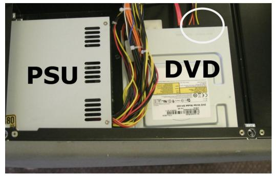
Remove the optical drive screws from the underside of the unit, and retain them for later. Remove the drive from the console.
