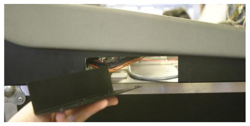
Use a cable-tie to secure the unused optical drive power connector to the rest of the loom as shown below.
