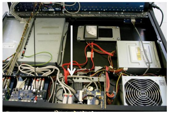
Locate the motherboard (at the rear of the console, indicated by the arrow above).
