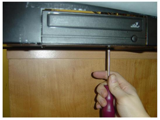
Install the optical drive blanking plate (1374-0090AB) from the inside. Fix it to the base of the chassis using the two optical drive screws.
