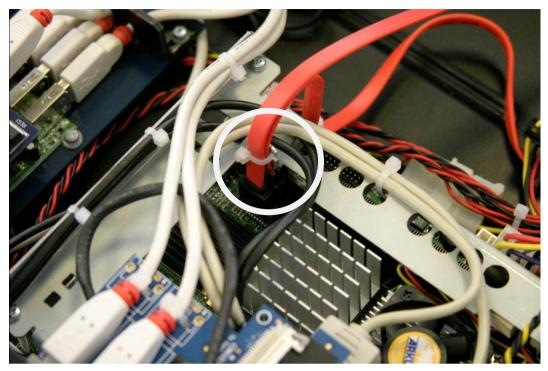
Locate the SATA cables connected to the motherboard (indicated above). Snip the cable tie connecting the two cables together.
