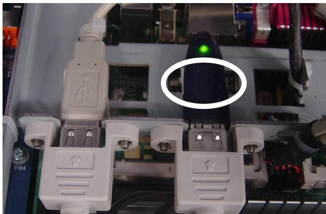
4. Locate the USB hub and remove the plastic comb (two screws)
