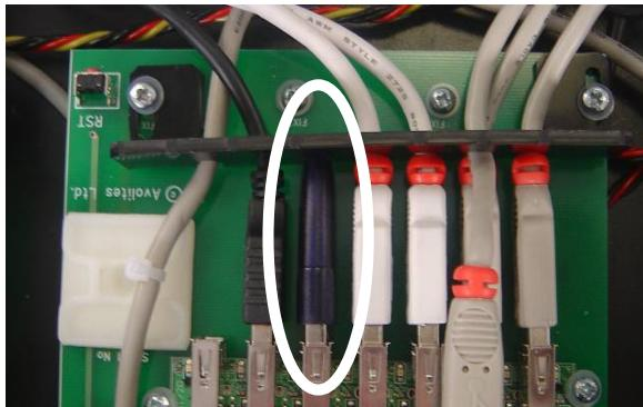
8. Replace the comb so it locks all USB cables and the dongle (See above) and tighten with two screws
