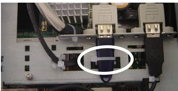
6. Locate the centre USB hub and remove the plastic comb (two screws)
