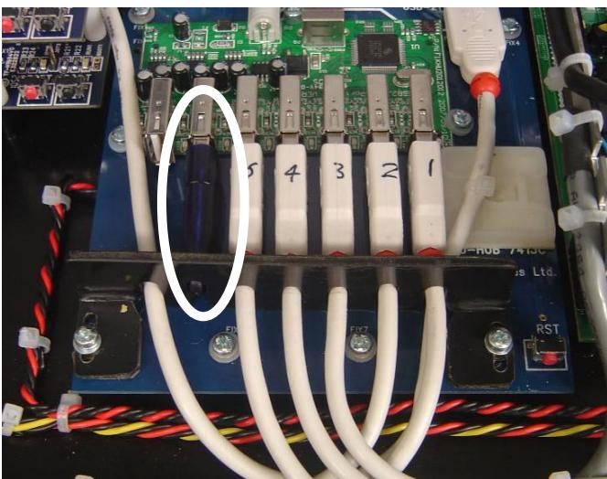
6. Replace the comb so it locks all USB cables and the dongle (See above) and tighten with two screws
