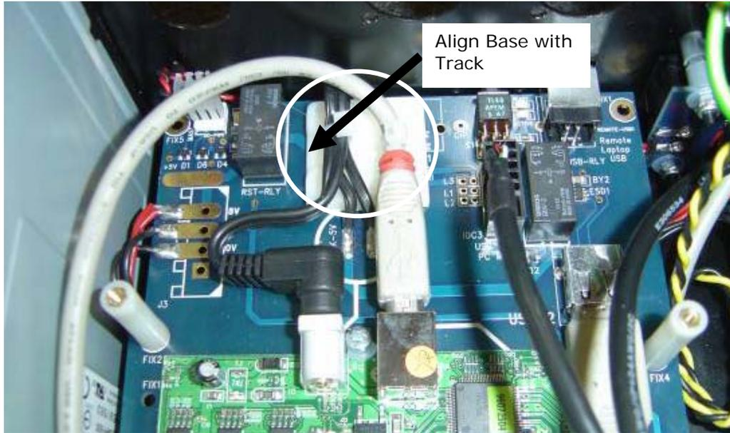
7. Wait for the area to be dried and then fit the cable tie base and press down. Position the cable tie base so it is aligned with the track on the PCB see arrow in picture above.
