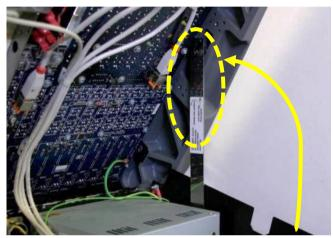
A. Locate the USB2 ports on Commell LV-67H motherboard, this can eb found near the SSATA cables as shown below
