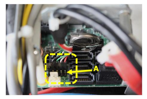
B. Insert 1x5 way connector from the supplied <u>1x5way to USB Type A cable</u> to the motherboard port with the Red wire to the right (next to SATA ports)
