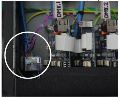
9. Titan Net Processor closing Plug lid earth wire back in, replace the lid and fix using the 8 screws previously removed (3x M4x8 screws with cap washers on each side of the lid and 2x M3 CSK screws on top of the lid)
