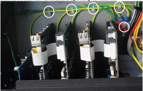
8. Plug the two RJ45 connectors and 3way mascon connector going into the TNP 7330 Ethercon board back in, such that the numbers match the printing on the front panel (Ethernet 1 on top).
