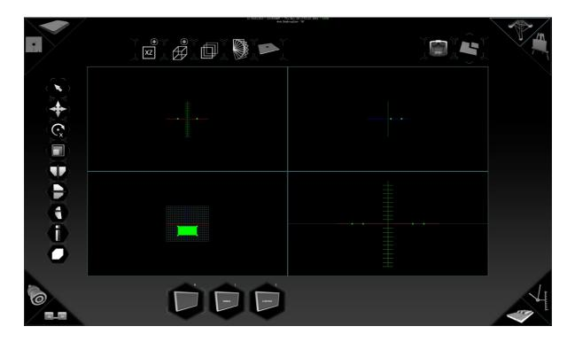
The modelling page itself is a sub window of the Stage Construction page – to access it, first click on the truss icon ( Stage Construction page ) and then look to the top right of the interface for the icon that looks like a square with one corner cut out and give it a click. Many of the functions and icons on the surface modelling page are carried across from other areas of Ai, so will seem familiar or obvious, but just to be sure, lets run through them all.
