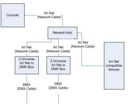
Once the system is connected together, the different outputs (or Nodes) can be configured.
